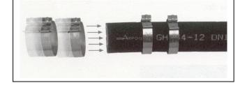
Step 5. Snap the cage into the groove on the nipple. The arms should extend over the hose length. When the cage has been correctly installed in the cage groove, the cage will be able to rotate in the groove. This step MUST be performed to ensure:
